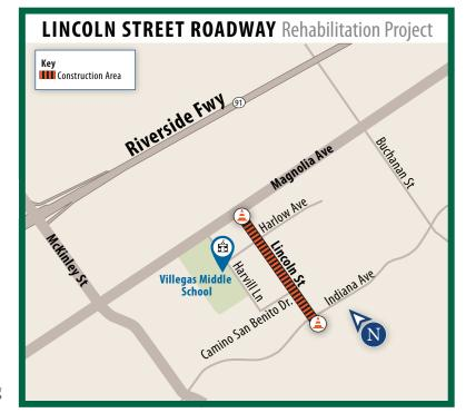
Construction crews started with utility relocation work to be followed by concrete work including cross gutters, curb and gutter improvements, and ADA ramp improvements. Next, crews will remove pavement and repave Lincoln Street, followed by street striping and signage installation.
