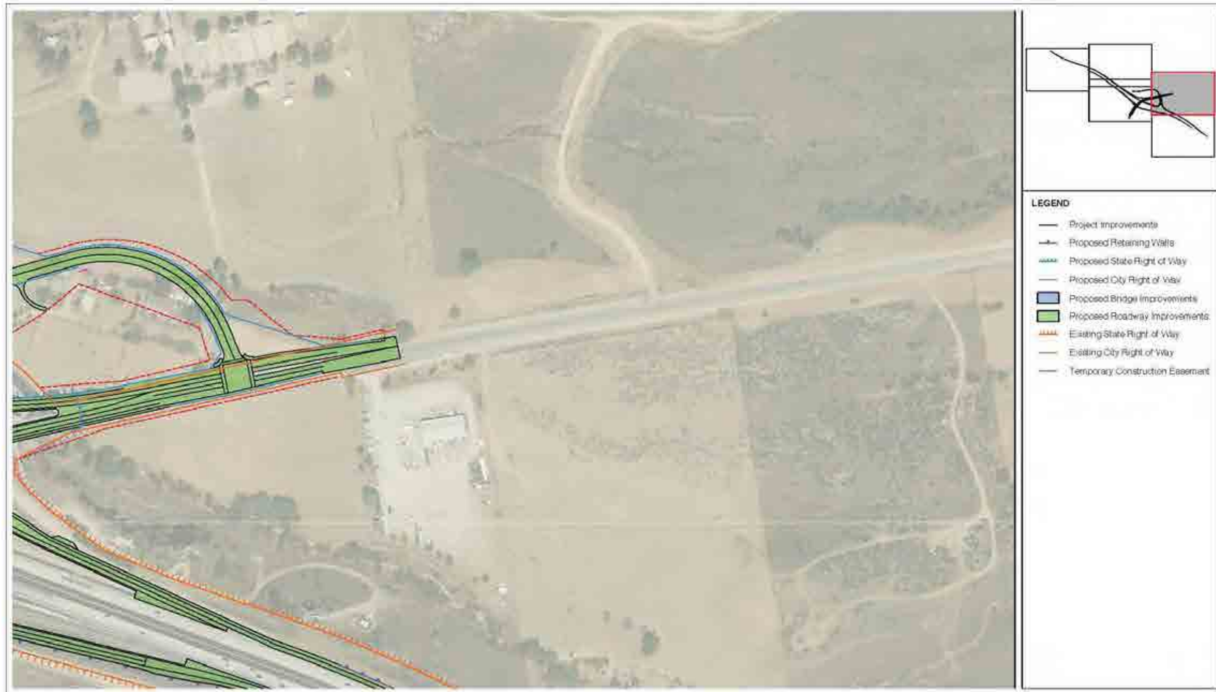
Figure 1-5d: Build Alternative 4 (Partial Cloverleaf)
